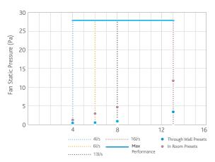
Tested through the wall with 300mm rigid duct and a low resistance grille.
