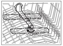
Wash the spray arm under running water. Use a thin pointed tool, e.g. a toothpick, to remove particles of soil from the holes.
