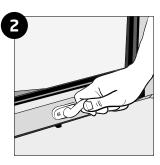
Close the bottom handle with the sash in the open position.
