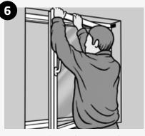
Insert the sash into the frame and carefully apply downward force (for three handled and one handled tilt and turn windows depending on size). This will remove any slackness in the glass packing and fittings which effectively reduces future wear and tear
