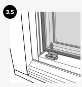
Remove the glazing bead clips from the sash using a screwdriver
