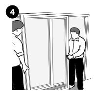
To re-install the door carefully replace the door leaf into the frame positioning the top of the door and bringing the bottom of the door in-line with the rollers.
