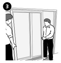
Lift the bottom of the door out at an angle and store safely to one side.
