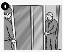
Remove door from frame Do not attempt this on your own. Observe health and safety guidelines at all times. Remove door from frame by opening to approx 300mm then lift door leaf up and out. Store
