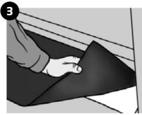
If the base is of a concrete construction, a DPC must be placed under the whole length of the threshold. Place door onto a bed of mastic
