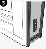
On adjacent frame, fix gasket to edge, top and bottom as shown. If available, fix 2mm spacer at top and bottom and at subsequent 500mm centres.
