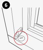
An adjustment screw is located in the bottom of the frame should the need arise to ease the sash in place after installation settle-
