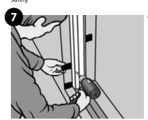
Check levels and fixings Refit the door and re-fasten all the screws checking that fixings are the correct distance apart
