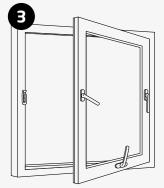
Return the sash to the closed position then open to the cleaning position.
