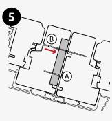
Secure with specified fixing at position (B)
