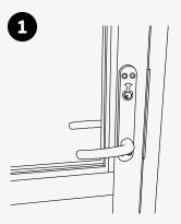
Cylinder: The cylinder is factory lubricated, however to maintain smooth operation and long life expectancy of cylinder and keys, it is recommended to lubricate the cylinder twice yearly. Use silicone spray.
