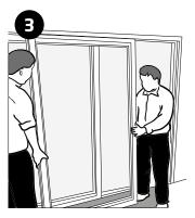
Lift the bottom of the door out at an angle and store safely to one side
