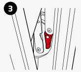
Turn the blowback restrictor to its origin. Now the sash can operate in ventilation position only. The lock however can be "burst" by an adult if sufficient force is applied in the case of emergency egress.
