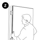
Lift the door blade off the hinges and store safely - Note If an overhead closer is installed unscrew & remove prior to lifting the door blade.
