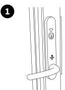
The door handle operates the multi-point locking mechanism to secure your door in place
