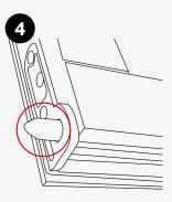
Lower the bottom handle to reveal the locking bullet at the end of the sash, apply recommended lubricant to this, any excess must be wiped off immediately
