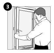
Release the sash from the bottom hinge side corner in the frame
