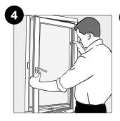
Tilt the sash inwards by appromately 30° then lift it up and away from the ball fitting located at the bottom of the 'hinged' side.
