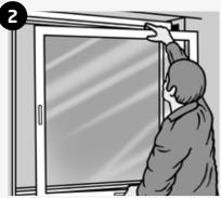
Remove sash if the window is inward opening. It is not recommended that outward opening sashes are removed
