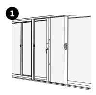
Open the sliding part of the door fully until it hits the closer.
