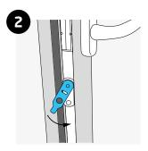
Press down the lifting mishandling device if mounted.
