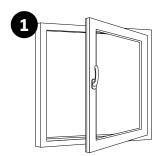
Open the window into the clean/ turn position by turning the handle to 180°
