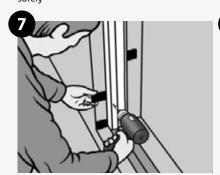
Check levels and fixings Refit the door and re-fasten all the screws checking that fixings are the correct distance apart
