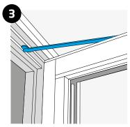
A friction stay may be installed on your door which can be activated by lifting the handle up when the door is open.
