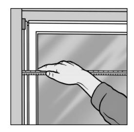
Check the rebate widths are equal across the hinge and locking points.
