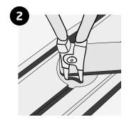
One operative needs to release [push apart the springs] on the centre sash casting. While the other holds the sash at 90°
