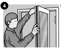
Remove door from frame Do not attempt this on your own. Observe health and safety guidelines at all times. Remove door from frame by opening to approx 300mm then lift door leaf up and out. Store safely
