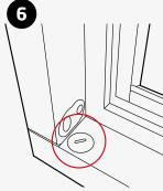
An adjustment screw is located in the bottom of the frame should the need arise to ease the sash in place after installation settlement.
