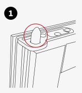
Open the window to the ventilation position and push down the two side handles to reveal the locking bullets at the head of the sash. Apply recommended lubricant on these, any excess must be wiped off immediately.
