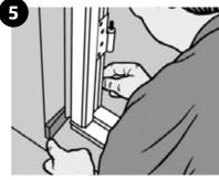
Place the frame in the opening, securing firstly with rot-proof dense wedges
