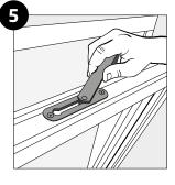
Disengage the stay on the top rail of the sash, by sliding the sash to the hinge side of the window.
