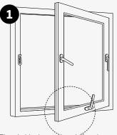
The wind-brake restrictor is found at the bottom of the frame when window is open in cleaning position.
