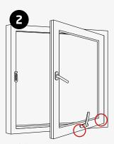
Carefully apply recommended lubricant at the restrictor stay at the head and ball /sockets at the 'hinged' corner.
