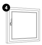
To secure the sash from falling out. Rotate the handle into turn position and close the sash
