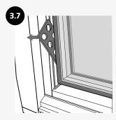
Remove glazing packers from the top and sides, marking their locations, leave the bottom packers until the glass is removed
