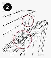
With the window still in the ventilation position, apply recommended lubricant at the restrictor stay, any excess must be wiped off immediately.
