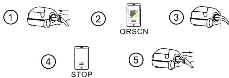
APP/RFID mode operation process flow
