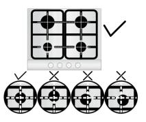
This appliance must only be used for the purpose for which it is intended, domestic cooking, and any other use will be considered improper and could therefore be dangerous. The Manufacturer will not be responsible for any damage or loss resulting from improper use. Before using burner, be sure, grid perimeters centre the burner as above figure.
