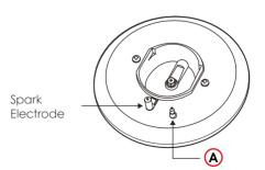
In case of flame failures of the burners for any reason, the flame failure sensor (A) will cut off the gas flow after a few seconds.
