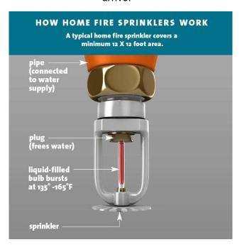
Because the water immediately cools the hot fire gases, only the sprinkler nearest the fire will activate. If, however the fire is hot enough that one sprinkler cannot handle it alone, hot gases will reach the next nearest sprinkler. That sprinkler would then activate to help stop the fire. This design of operation limits the number of sprinklers needed to stop a fire.
