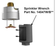
Step 1: Carefully slide the wrench sideways around the deflector and pins
