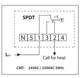
Wiring diagrams above are shown for heating applications.
