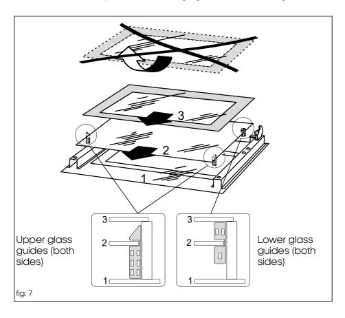
Important: Do not disassemble the door without it having been removed from the oven. Weight differences could cause the door to snap shut, causing damage to the oven and/or the user.
