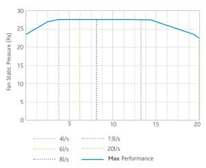
Tested through the wall with 300mm rigid duct and a low resistance grille.
