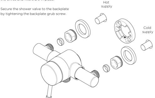
**Note:** The shower valve inlet positions are shown at the rear as an example.
