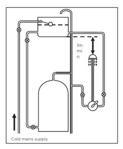
Important: If you install this shower valve with a gravity fed system, there must be a minimum head (vertical distance) from the underside of the cold water storage tank to the showerhead position of at least 1 metre.
