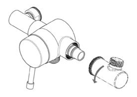
Unscrew small elbow anti-clockwise
